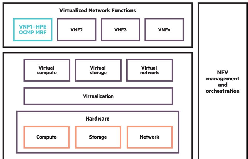
Figure 4: HPE OCMP MRF as a VNF in the ETSI NFV reference model
