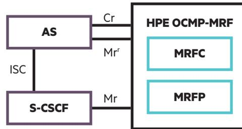
Figure 1: HPE OCMP MRF in 3GPP IMS as per TS 23.218
