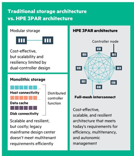
Figure 1. Traditional storage architecture vs. HPE 3PAR architecture
