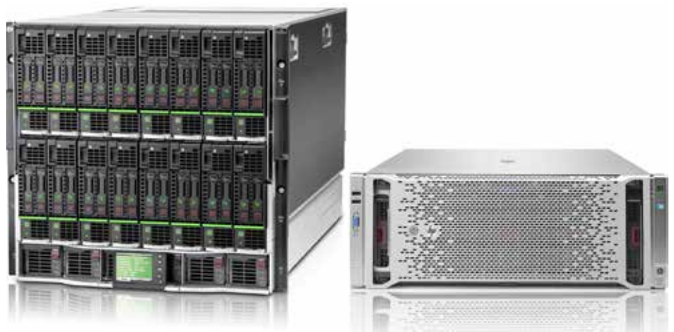
Figure 4. HPE BladeSystem c7000 enclosure with server blades + DL580 Gen8 rackmount server
