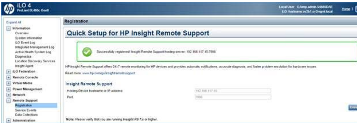
Figure B-3. Host IP address and port is that of the SIM CMS
