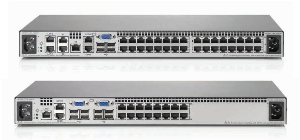
The HPE IP Console Switch G2 with VM and Server Console Switch G2 with VM integrated keyboard, video, and mouse (KVM) capabilities and serial access into a single management console for all your servers, network devices, and technology infrastructure
