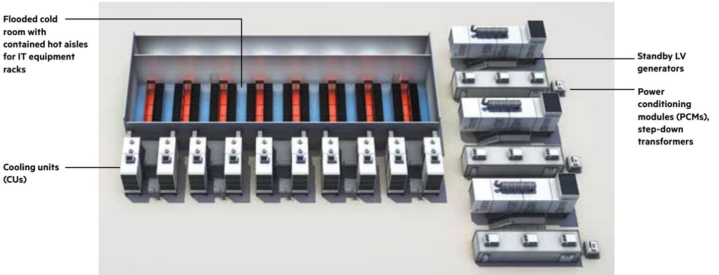
Figure 6: Mechanical and electrical systems
