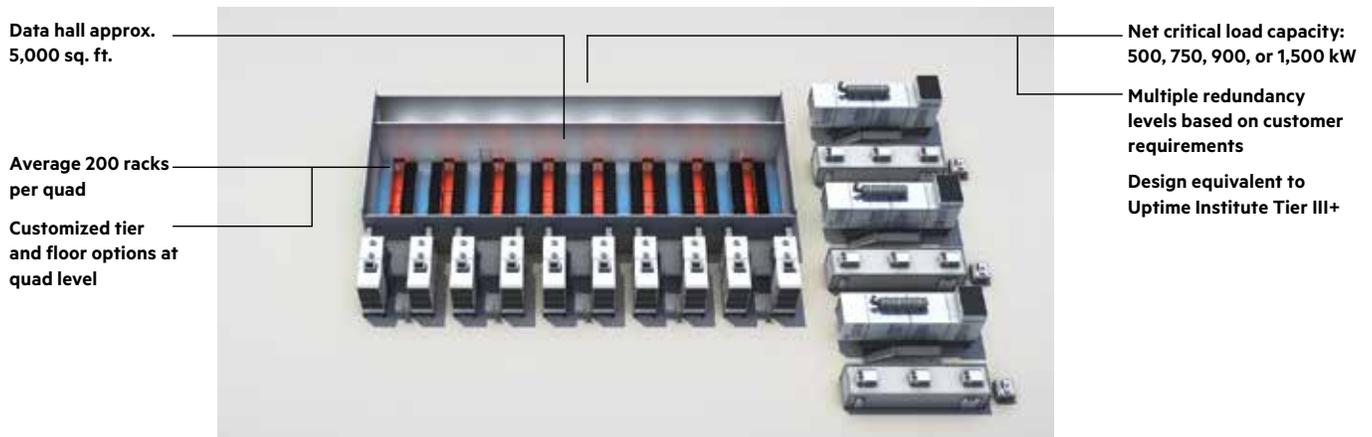
Figure 3: Details of a quadrant
