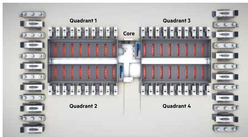
**Figure 2:** The FDC building consists of a central core surrounded by up to four quadrants
