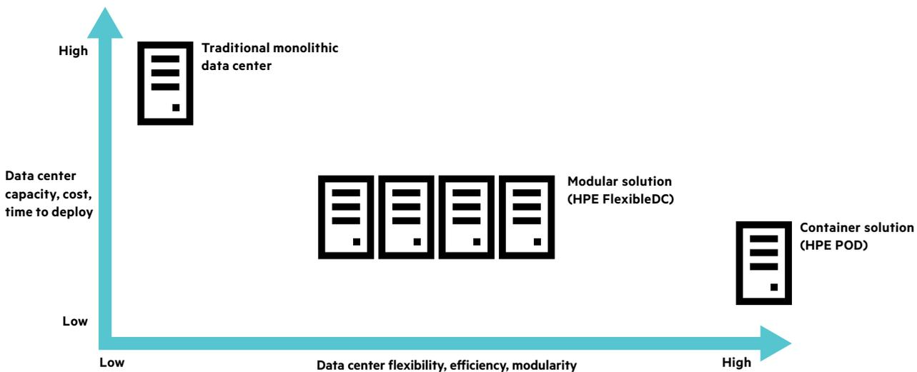
Figure 1: Levels of modularity
