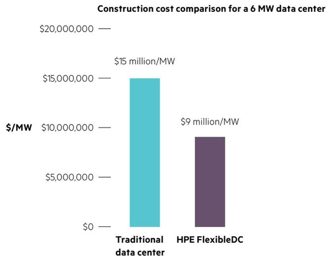
Estimated costs for a data center with 6 MW of IT load. Costs for the traditional monolithic data center are based on "The Economics of Prefabricated Modular Data Centers," 451 Research, May 2012; costs for the modular DC are based on Hewlett Packard Enterprise research.
