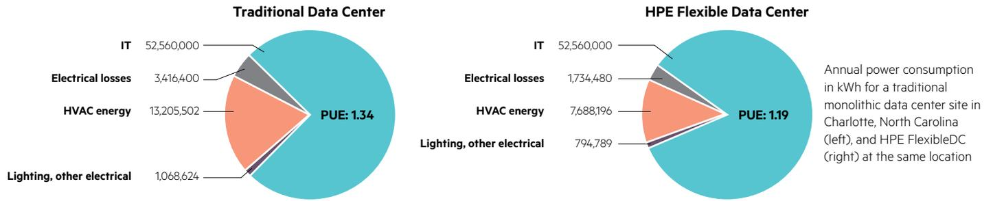
Figure 8: FDC offers lower energy consumption and a better PUE compared to the traditional data center
